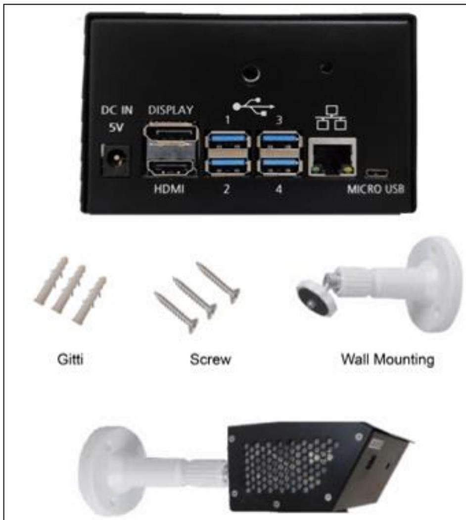
1. Fix wall mounting on wall with the help of screws & Gitti
